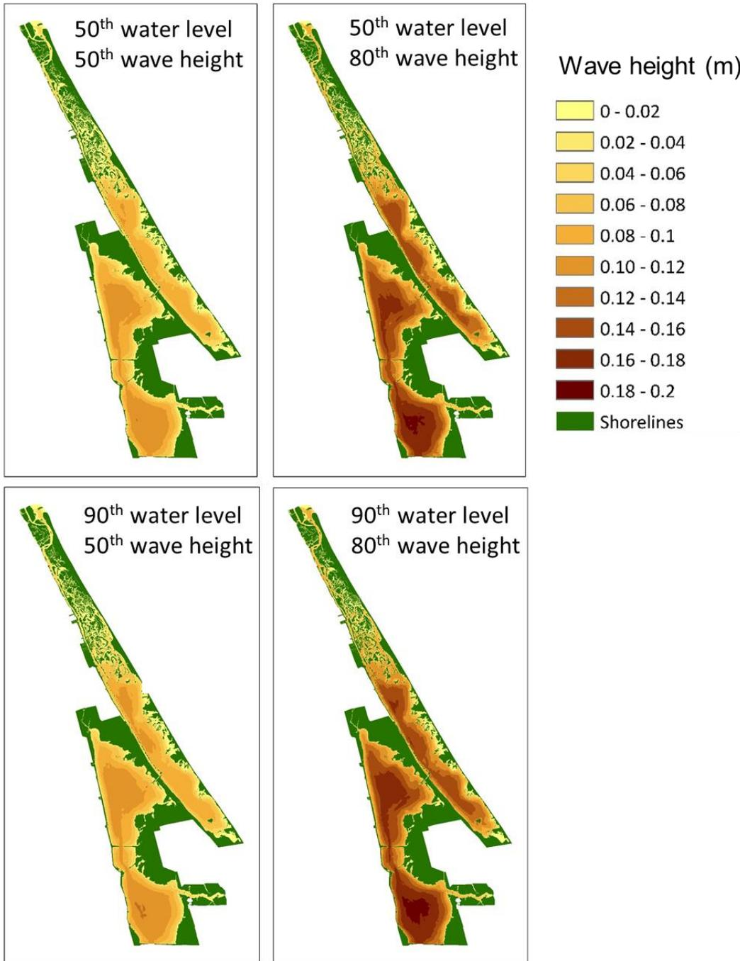
Figure 4. Modelled wave heights over the study area: 50<sup>th</sup> and 80<sup>th</sup> percentile wave heights in meters, modelled with 50<sup>th</sup> and 90<sup>th</sup> percentile water levels.
