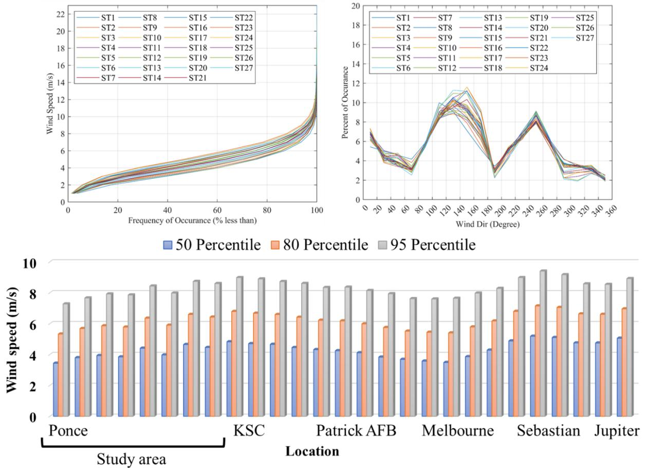
Figure 3. Wind speed and direction frequency distributions from Ponce de Leon Inlet (ST1) to Jupiter Inlet (ST27). Distributions of wind speed and direction vary little over the study area and IRL in general.
